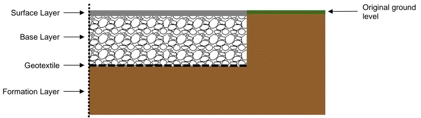
If the ground is soft or wet, the path is usually built-up above ground level to prevent water running back on to the surface. In the diagram below, you will see that the surface layer now sits above the original ground level. We call this a **half tray**.
